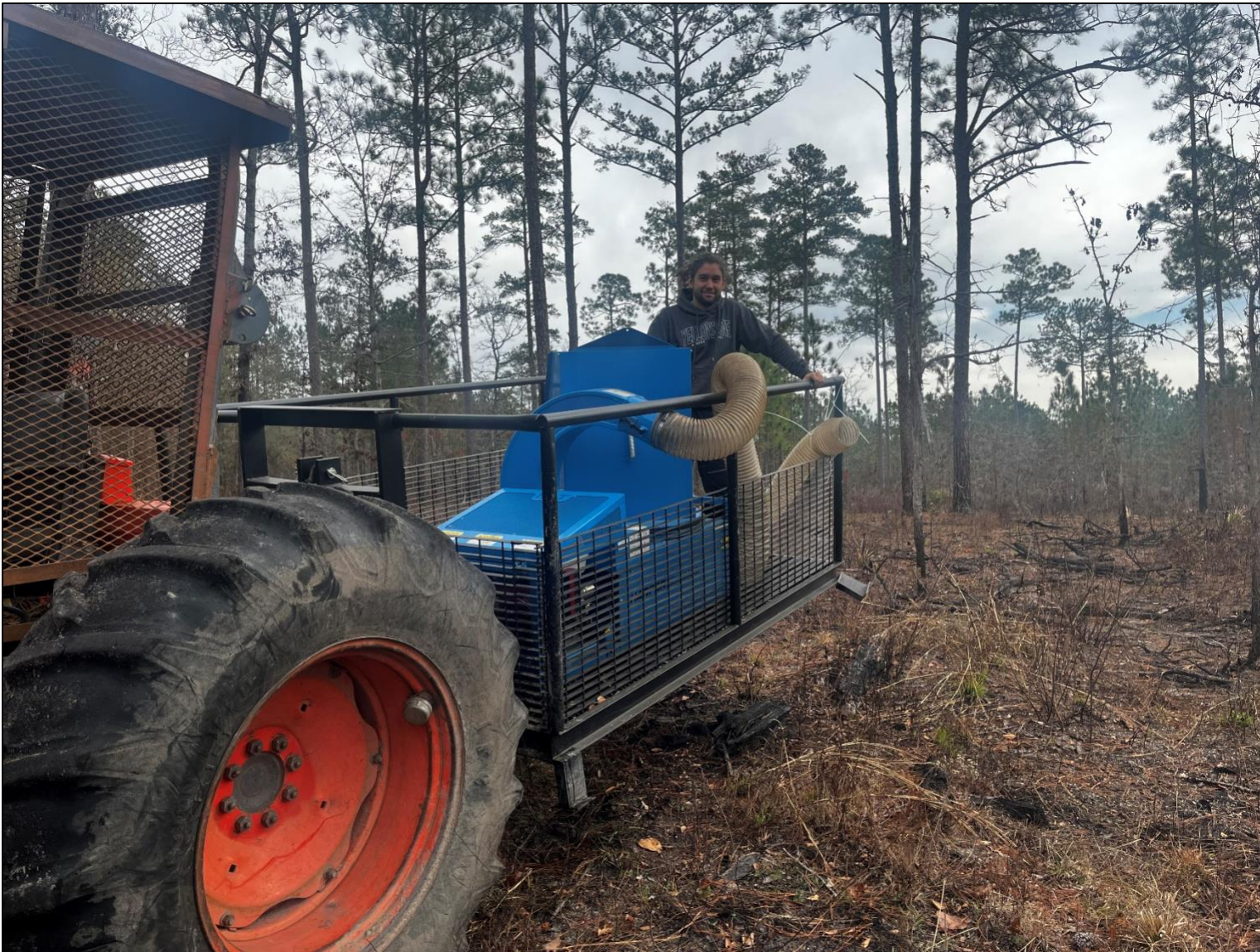
Photo 4: Crewmember on a platform with a hay blower borrowed from our partners at Georgia Department of Natural Resources. The hay blower receives seed into a large hopper and uses a gas-powered motor to propel seed in the desired direction.
