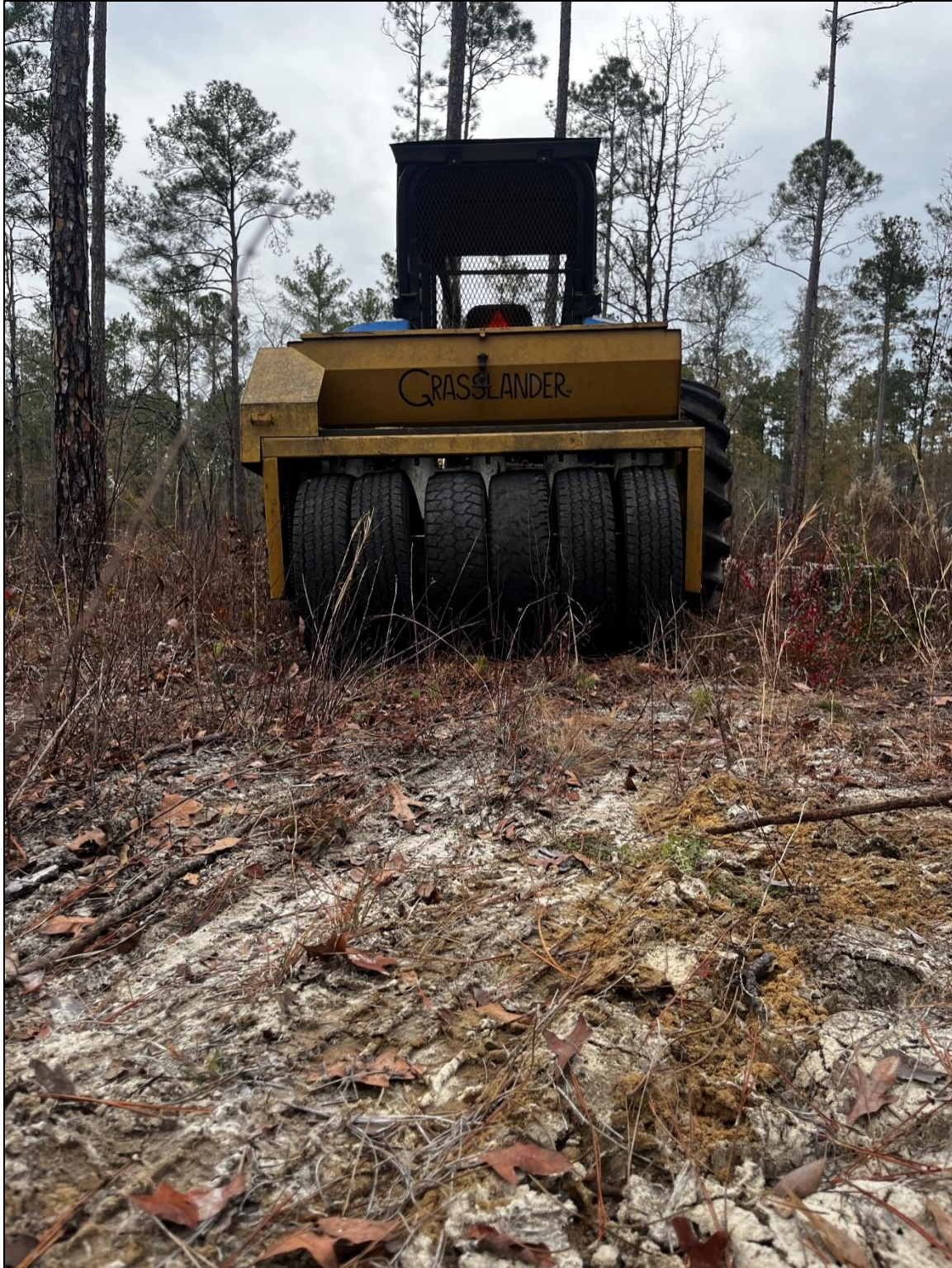
Photo 3: As the tractor passes through carrying the Grasslander™, metal tines lightly scratch the surface of the ground. As the tires move forward, a set of gears engage an agitator in the hopper that disperses the seed below, then the tires run over the seed to ensure good seed to soil contact.
